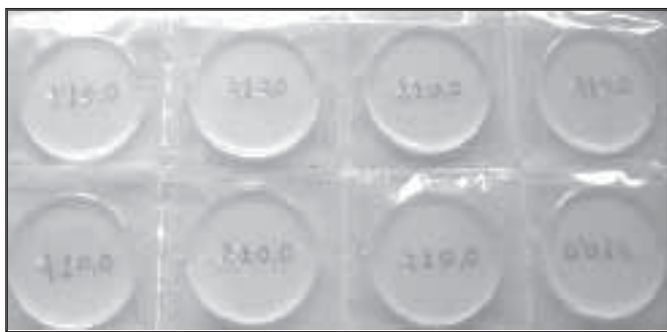
Figure 7. PVP Hydrogel membranes with 0.01% Laponite XLG irradiated with EB at 25 kGy
