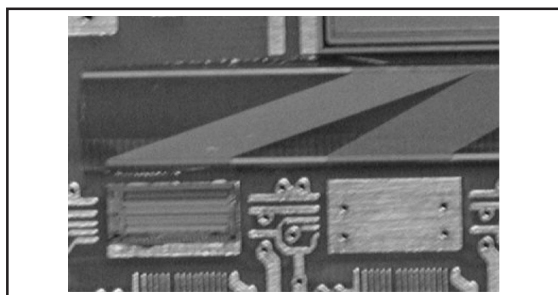
Figure 4. Detail of the pitch adapter (middle) which connects the detector (top) to each of the 6 RX64 ASICs (bottom).
