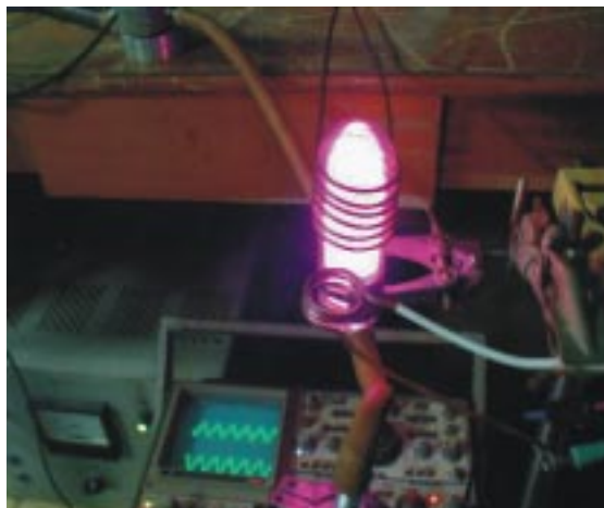
Figure 6. Plasma obtained in a test session. Antenna is coiled around the plasma chamber, an auxiliary antenna allows to observe a signal sample in the oscilloscope.
