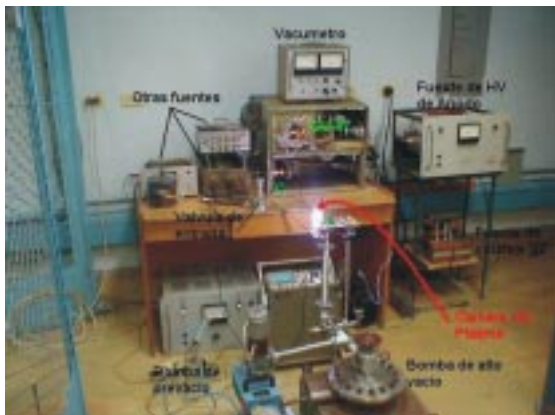
Figure 5. Test bench. Observe plasma chamber containing ionized gas, pre-vacuum pump, high vacuum pump, main amplifying stage, high voltage anode source, high voltage grid 2 source, gas supplying valve, other voltage sources, cooling system is hidden behind the main amplifying block.
